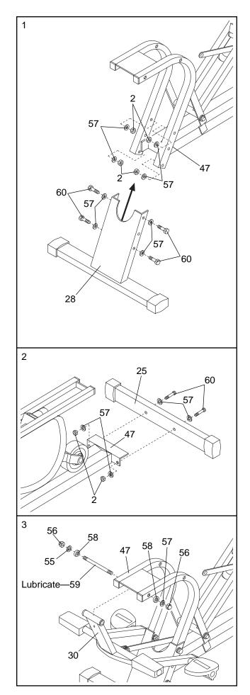
4. Lubricate a M8 x 157mm Axle (59). Attach the Handlebar Swing Arm (29) to the Main Frame (47) with the M8 x 157mm Axle, two M9 Rubber Shield Washers (58), two 5/16" Washers (55), and two M8 Acorn Nuts (56).
